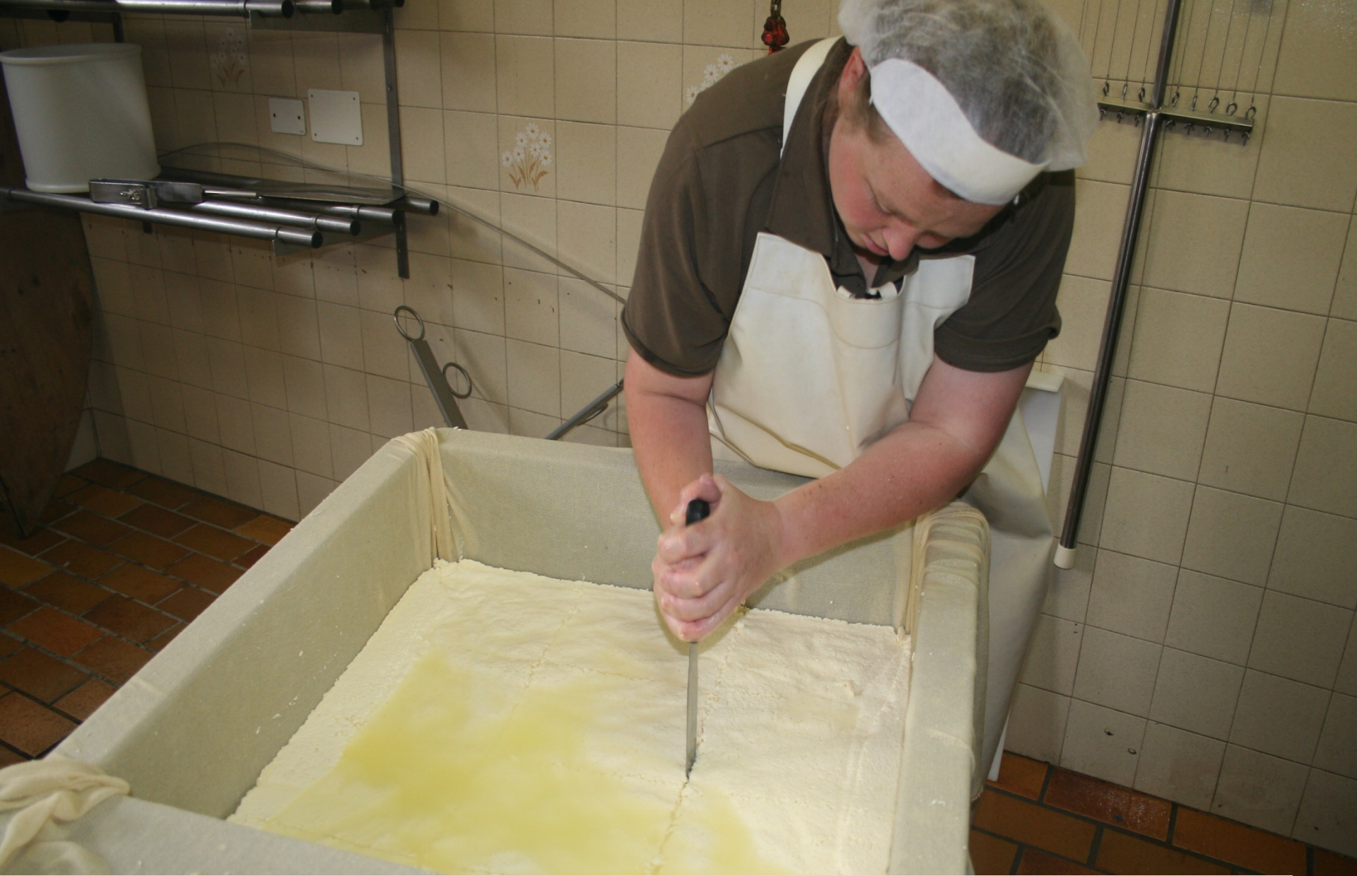
After the pre-pressing (5 min) cutting the pieces for forming in the cheese molds
